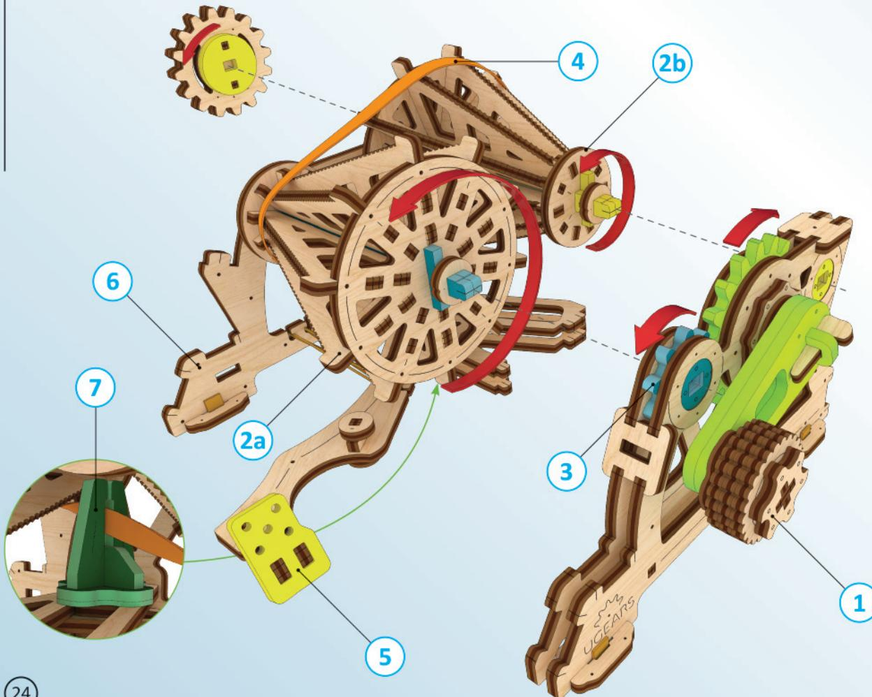
**ENG** Rotating the key (1) initiates the drive cone pulley (2a) via the reducer (3). The belt transfers the rotation to the driven cone pulley (2b). Pushing the pedal (5) attached to the body (6), the transmission fork (7) holding the belt moves, which changes the rotation speed of the driven cone pulley (while the drive cone pulley's speed remains the same).
